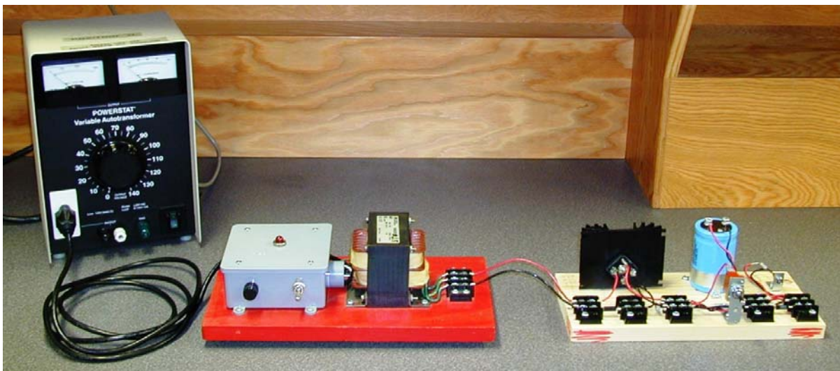
Circuit Layout Showing Variac, 25V Transformer, and DBR
