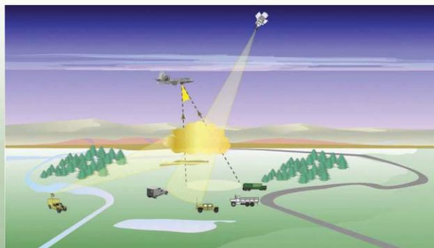
**[FIG1]** Standoff hyperspectral sensors can be deployed on satellites, unmanned aerial vehicles, and ground-based platforms.
