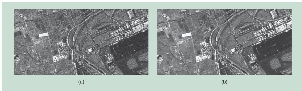
**[FIG3]** (a) The single-look TerraSAR-X image of Barcelona and (b) the radiometry estimated by the nonlocal method [11]. Images are  $511 \times 1,043$  pixels with a spatial resolution of 2.5 m. (Images used with permission of Infoterra GmbH.)
