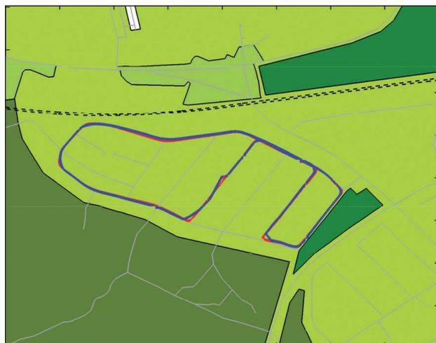
**FIGURE 7.** Ten routes were driven (red GPS line), and the position using map-aided position is depicted for one of them (blue line).
