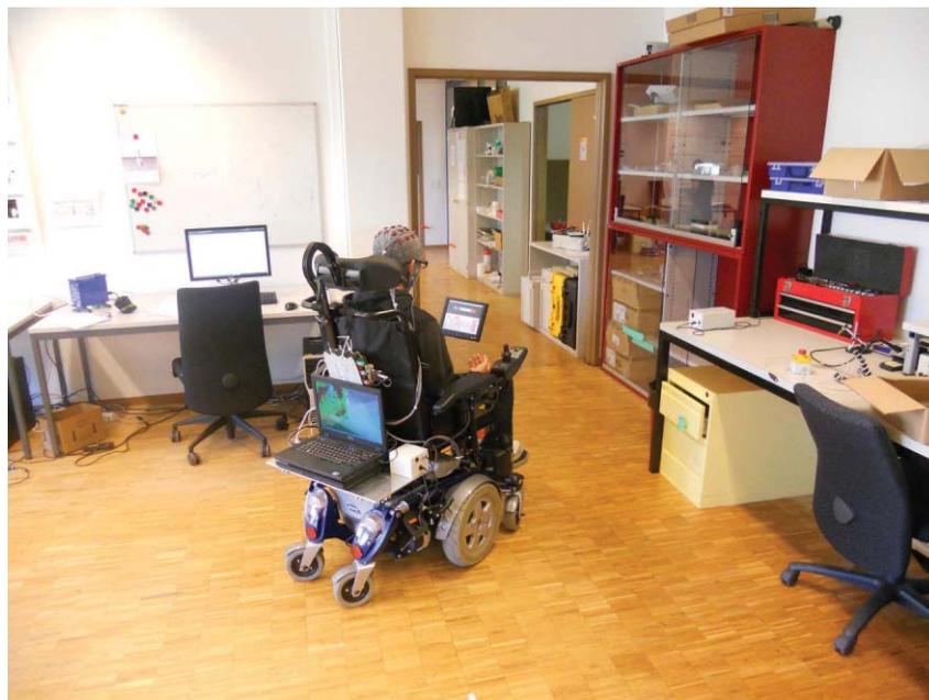
**FIGURE 1.** A robotic wheelchair equipped with a BCI that records neural signals and decodes them in order to transform user’s intentions into appropriate commands. (Photo courtesy of Ecole Polytechnique Fédérale de Lausanne’s Defitech Foundation Chair in Brain-Machine Interfaces.)
