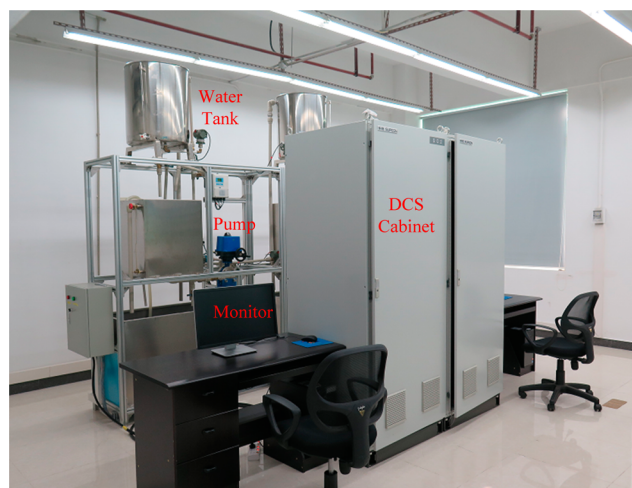
Figure 7. Water tank control system.
