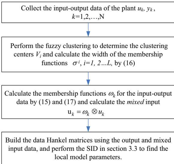
Fig. 1. Procedure of the data-driven fuzzy modeling.
