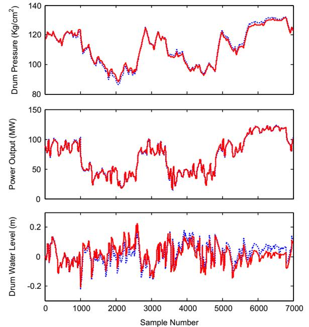
Fig. 3. Fuzzy model identification for the boiler-turbine unit (solid-red: estimated outputs; dotted in blue: real outputs). (For interpretation of the references to color in this figure legend, the reader is referred to the web version of this article.)
