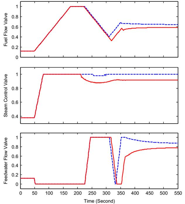
**Fig. 9.** Performance of the boiler-turbine unit in the CCS mode: Manipulated Variables (solid in red: FMPC\_S; dashed in blue: linear\_MPC\_S). (For interpretation of the references to color in this figure legend, the reader is referred to the web version of this article.)
