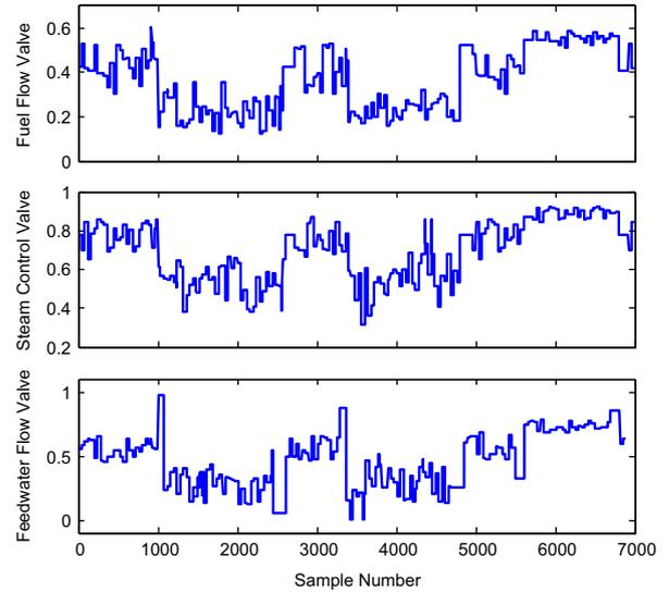
Fig. 2. Input signals used in the fuzzy subspace identification method.
