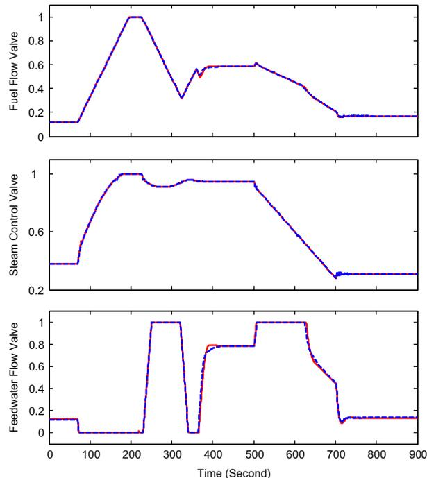
**Fig. 11.** Performance of the boiler-turbine unit in AGC mode: Manipulated Variables (solid in red: DDFPC; dotted in blue: FMPC\_S). (For interpretation of the references to color in this figure legend, the reader is referred to the web version of this article.)
