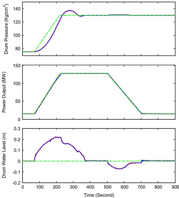
**Fig. 10.** Performance of the boiler-turbine unit in AGC mode: Output Variables (solid in red: DDFPC; dotted in blue: FMPC\_S; dot-dashed in green: reference). (For interpretation of the references to color in this figure legend, the reader is referred to the web version of this article.)
