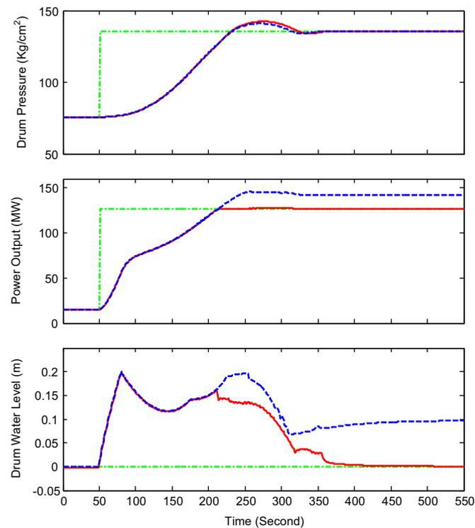
**Fig. 8.** Performance of the boiler-turbine unit in the CCS mode: Output Variables (solid in red: FMPC\_S; dashed in blue: linear\_MPC\_S; dot-dashed in green: reference). (For interpretation of the references to color in this figure legend, the reader is referred to the web version of this article.)
