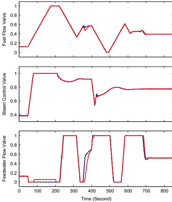
**Fig. 7.** Performance of the boiler-turbine unit in the CCS mode: Manipulated Variables (solid in red: DDFPC; dashed in blue: FMPC\_S; dotted in black: FMPC\_T). (For interpretation of the references to color in this figure legend, the reader is referred to the web version of this article.)
