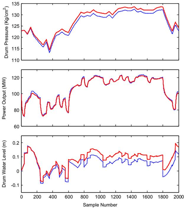
Fig. 5. Fuzzy model verification in the medium-high power region (solid in red: estimated outputs; dotted in blue: real outputs). (For interpretation of the references to color in this figure legend, the reader is referred to the web version of this article.)
