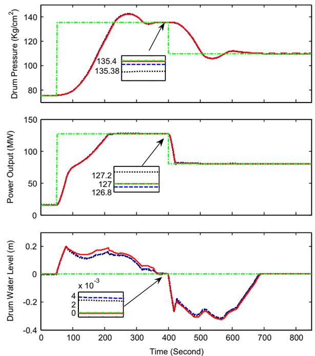
Fig. 6. Performance of the boiler-turbine unit in the CCS mode: Output Variables (solid in red: DDFPC; dashed in blue: FMPC\_S; dotted in black: FMPC\_T; dot-dashed in green: reference). (For interpretation of the references to color in this figure legend, the reader is referred to the web version of this article.)
