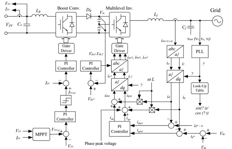
Fig. 3. Control block diagram of a 3-level NPC inverter system.
