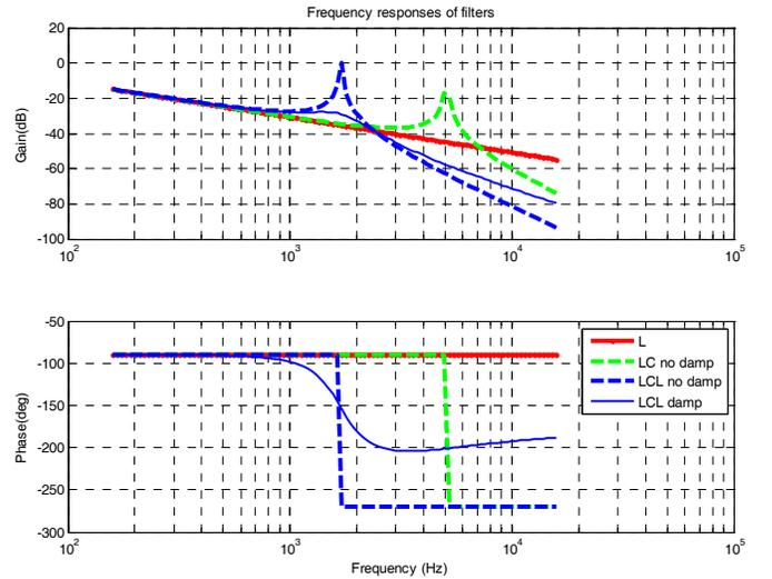
Fig. 5. Bode plots of the LC filter.
