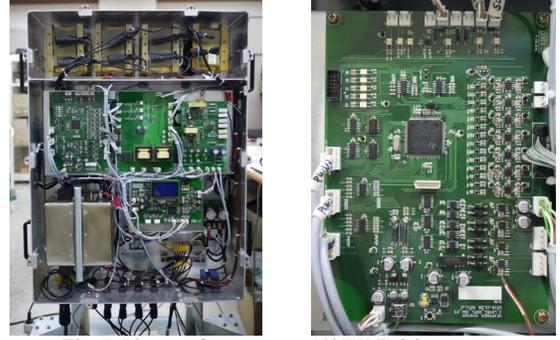
Fig. 7. Photos of a prototype 13kW NPC inverter.
