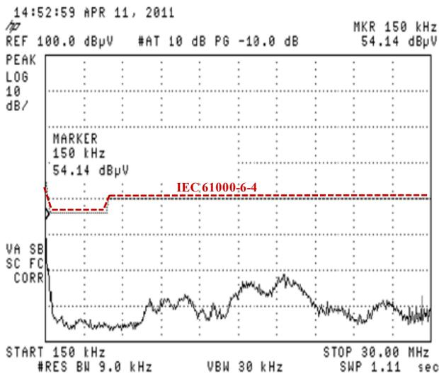
Fig. 11. Conducted noise measurement of the proposed inverter system.
