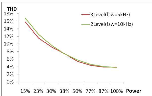
(b) Comparison of THDs of injected current to the grid.
