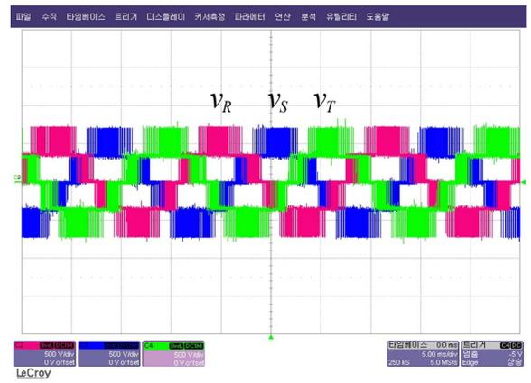
Fig. 8. Experimental three-level NPC inverter output voltage waveforms ( $v_R$ ,  $v_S$ , and  $v_T$ )
