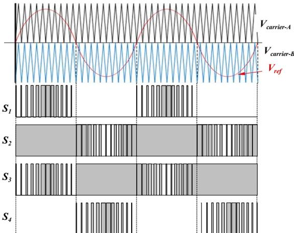
Fig. 2. PD PWM switching pattern of one 3-level inverter phase-leg.
