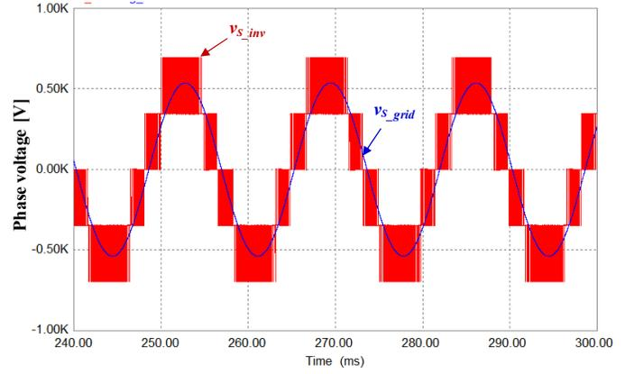
(b) Grid voltage and 3-level PWM output voltage.
