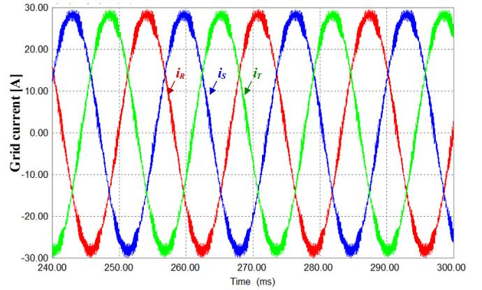
(c) Injected current to the grid ( $I_r$ ,  $I_s$ ,  $I_t$ ).
