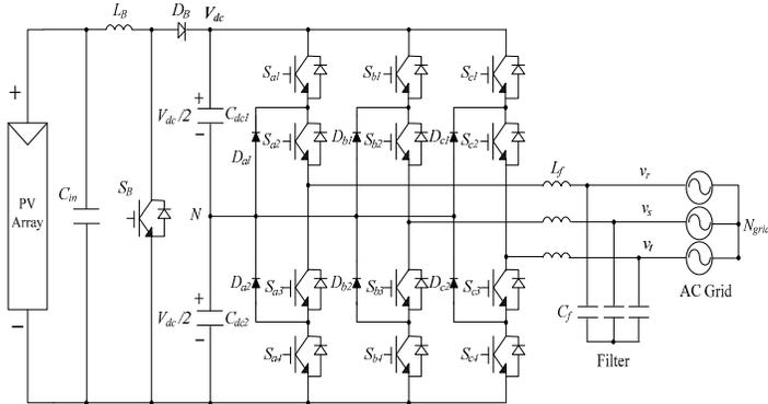
Fig. 1. Overall configuration of a transformerless three-phase 3-level NPC inverter system.
