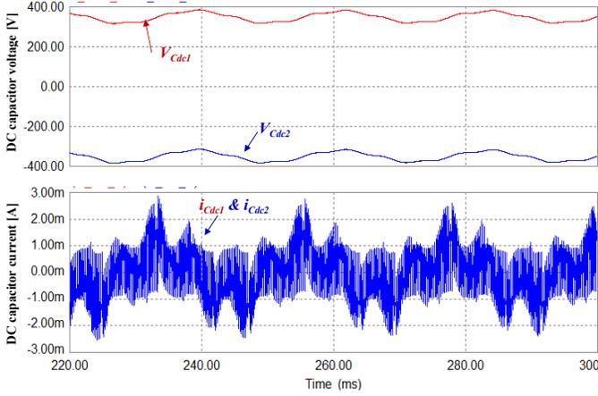
Fig. 6. Voltages (top) and currents (bottom) of the parasitic capacitors between PV terminals and the ground.
