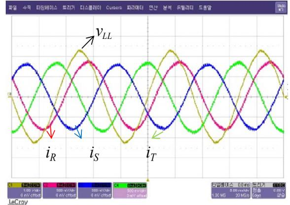
Fig. 9. Experimental waveforms of grid voltage  $V_{LL}$  and current  $i_R$ ,  $i_S$ ,  $i_T$  at rated output.
