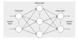
A Feedforward Multi-layer Network: each circle corresponds to a node and each arrow represents a weighted link.
