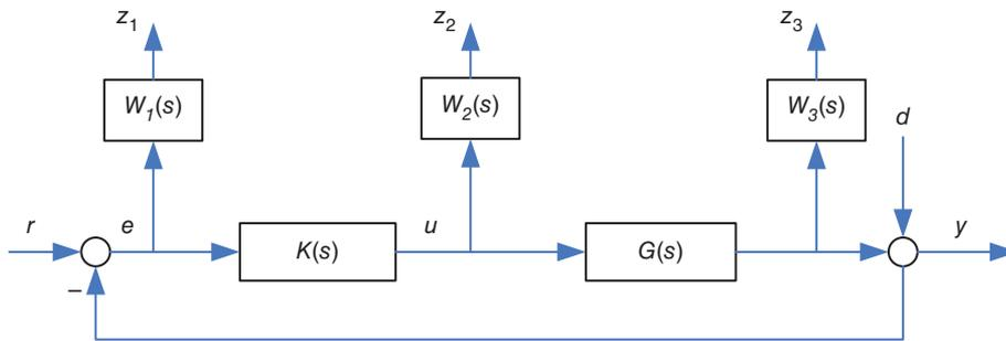
FIGURE 13 | Block diagram of a typical  $H_\infty$  mixed sensitivity problem.
