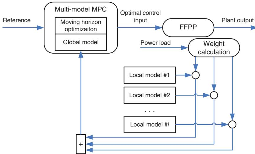
**FIGURE 15** | Control diagram of model-weighted multi-model MPC.
