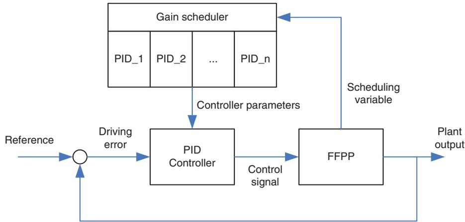
FIGURE 12 | Gain Scheduling PID control.
