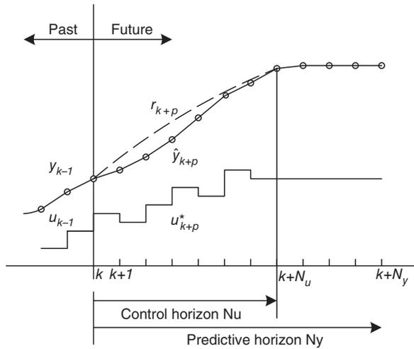
**FIGURE 14** | Basic working principle of the MPC.
