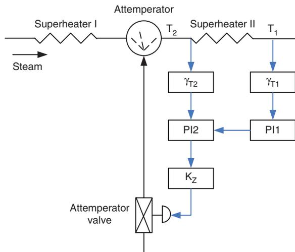
**FIGURE 10** | Classical cascade SST control in the FFPP ( $T_1$  is final steam temperature;  $T_2$  is the steam temperature signal immediately after the attemperation;  $\gamma_{T1}$  and  $\gamma_{T2}$  are the temperature transmitters;  $K_z$  is the actuator of the attemperator valve).
