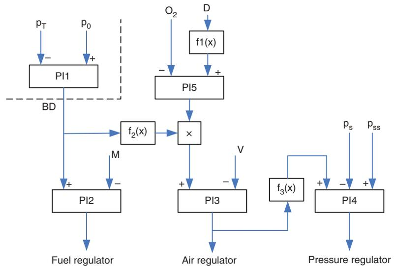
**FIGURE 7** | Three sub regulators of boiler combustion control system ( $P_0$ : main steam pressure set-point;  $P_T$ : main steam pressure output;  $D$ : main steam flow rate;  $O_2$ : oxygen content in the flue gas;  $V$ : air flow rate;  $P_{ss}$ : furnace pressure set-point;  $P_s$ : furnace pressure output;  $BD$ : boiler demand).
