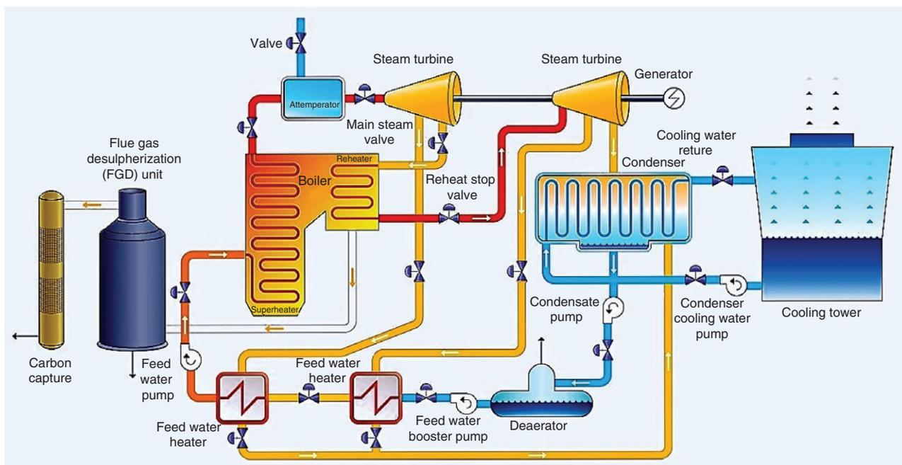
**FIGURE 2** | Simplified supercritical power plant (Picture from [http://www.flowserve.com/Industries/Power-Generation/Conventional-Steam/Flowserve-Products-Used-in-Supercritical-Units,en\\_US](http://www.flowserve.com/Industries/Power-Generation/Conventional-Steam/Flowserve-Products-Used-in-Supercritical-Units,en_US)).
