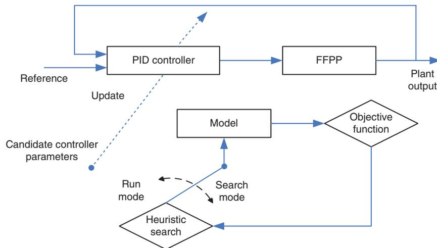
**FIGURE 11** | Block diagram of a typical tuning method for PI/PID parameters.
