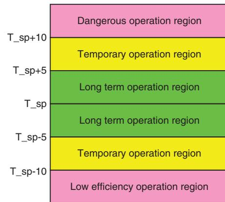
**FIGURE 9 |** Operation regions of superheater steam temperature ( $T_{sp}$  is the temperature set-point and the numbers represent temperature deviations in Celsius degree).
