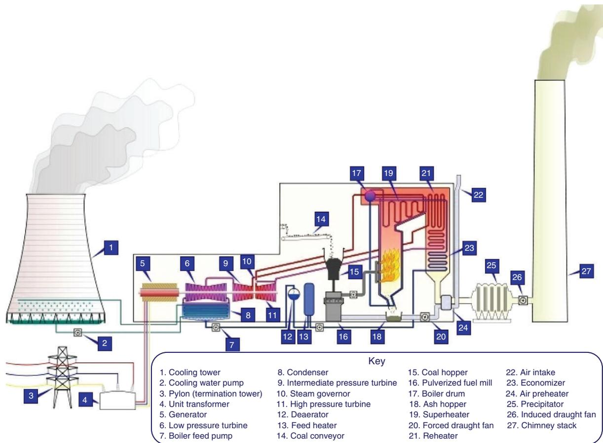
**FIGURE 1** | Simplified coal-fired subcritical power plant (Picture from [http://en.wikipedia.org/wiki/Thermal\\_power\\_station#Boiler\\_furnace\\_and\\_steam\\_drum](http://en.wikipedia.org/wiki/Thermal_power_station#Boiler_furnace_and_steam_drum)).
