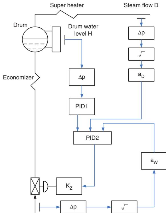
**FIGURE 8 |** Three elements cascade feedwater control system for a drum type boiler ( $\Delta p$  is the differential pressure transmitter;  $\sqrt{\quad}$  is the square root extractor;  $a_w$ ,  $a_D$  are the sensitive coefficients of feedwater flow rate and steam flow rate signals;  $K_z$  is the actuator of the feedwater flow control valve).
