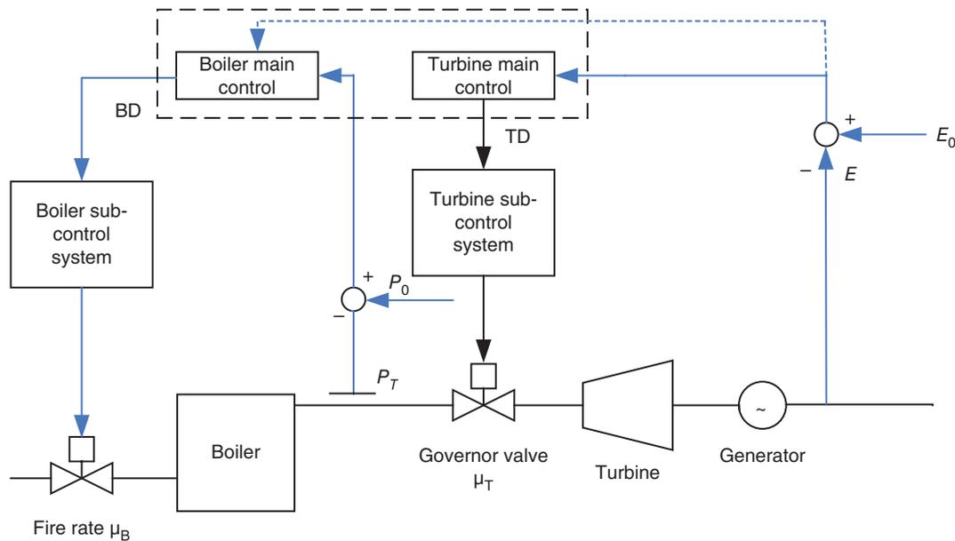
**FIGURE 4** | Working Principle of the Coordinated BF mode ( $E_0$ : load set-point;  $P_0$ : main steam pressure set-point;  $E$ : power output;  $P_T$ : main steam pressure output; BD: boiler demand; TD: turbine demand).
