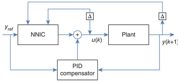
**FIGURE 18** | NNIC augmented by a PID compensator.
