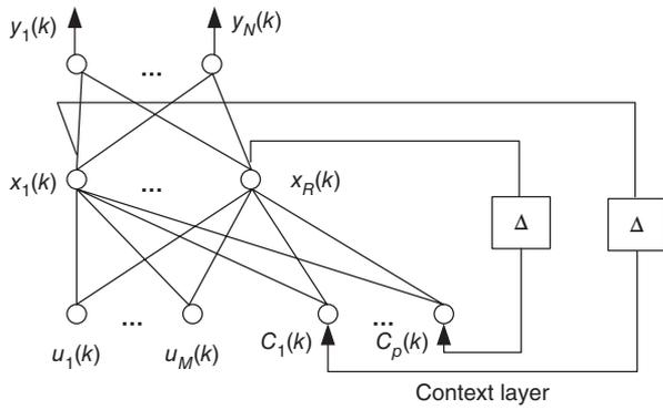
FIGURE 16 | Basic structure of the ENN.
