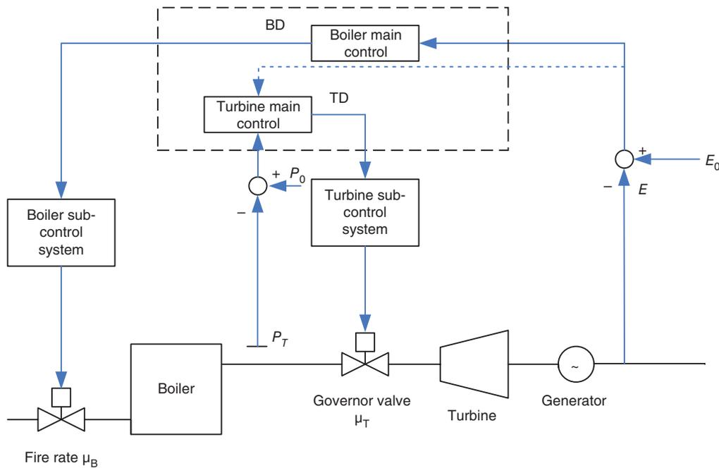
**FIGURE 5** | Working Principle of the Coordinated TF mode ( $E_0$ : load set-point;  $P_0$ : main steam pressure set-point;  $E$ : power output;  $P_T$ : main steam pressure output; BD: boiler demand; TD: turbine demand).
