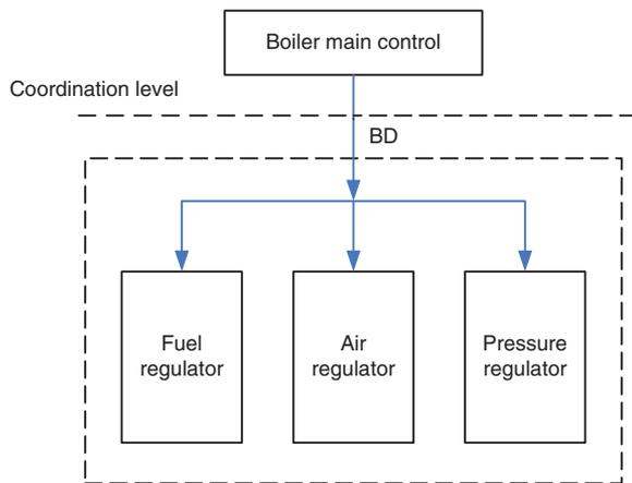
**FIGURE 6** | Combustion control system (BD: boiler demand).
