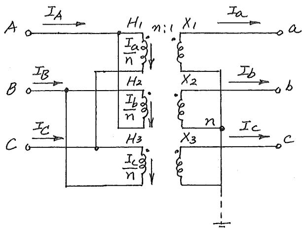
This time, we connect  $\Delta$  in high-voltage windings in the order of  $A - C - B$  ( $H_1 - H_3 - H_2$ ).
