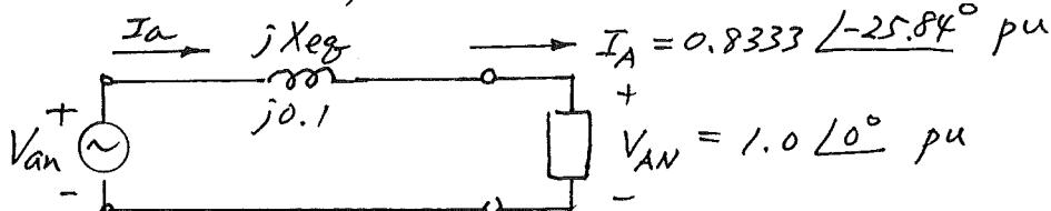
$$V_{an} = V_{AN} + (jX_{eg}) I_A = 1.0 \angle 0^\circ + (j0.1)(0.8333 \angle -25.84^\circ)$$
