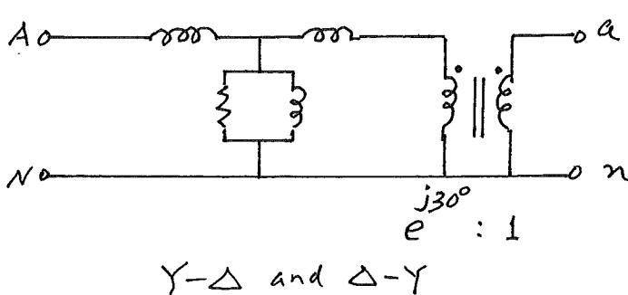
Furthermore, the per-unit impedance of the 3φ transformer is the same as the per-unit impedance of the single-phase transformer! (Why?)
