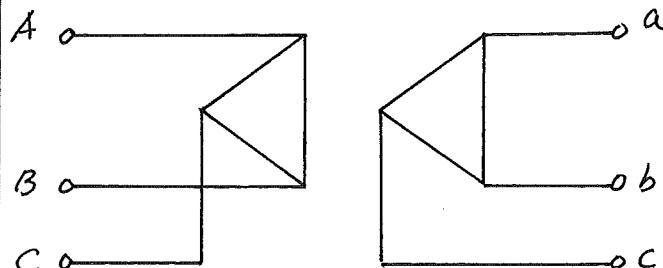
The  $\Delta-\Delta$  connection has the advantage that one phase can be removed for repair or maintenance while the remaining phases continue to operate as a three-phase bank. This open  $\Delta$  (or  $V$ ) connection permits balanced three-phase operation with the kVA rating reduced to 58% of the original bank. (Why?)
