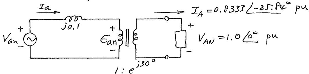
$$E_{an} = e^{-j30^\circ} V_{AN} = 1.0 / -30^\circ$$
