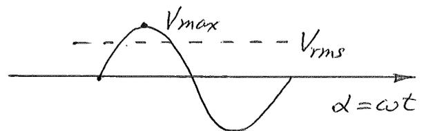
The rms value only account for the magnitude of the voltage. In order to account for the phase angle, we introduce the complex variable. Specifically, recall the Euler's identity:  $e^{j\phi} = \cos \phi + j \sin \phi$ . This suggests that the cosine term is the "real part" of the complex variable  $e^{j\phi}$ .
