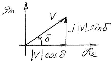
Phasor is a vector in the complex plane, which has magnitude  $V_{rms}$  and phase angle  $\delta$ .
