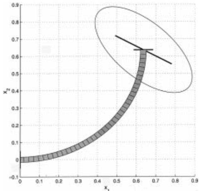
Fig. 6. For a one-section manipulator, the CME indicates a singular configuration (bold line) while the GME does not (thin line).
