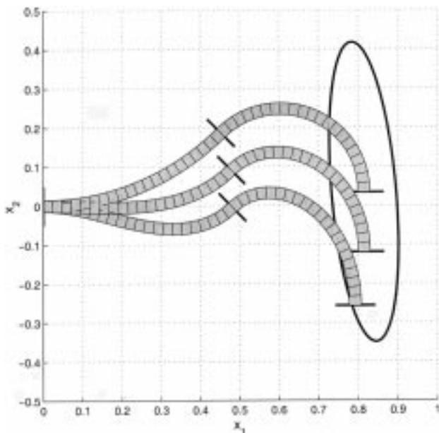
Fig. 9. A compliance ellipsoid indicates that the robot is more compliant to vertical forces on the end-effector than horizontal forces.
