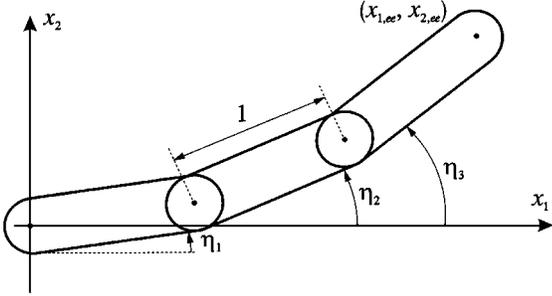
Fig. 4. Simple three-link manipulator.
