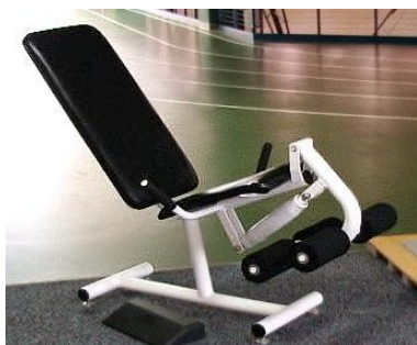
Figure 1: A leg extension machine with a linear hydraulic damper.
