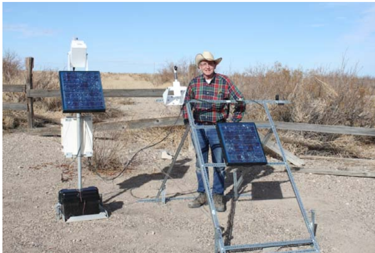
Rotating Shadow Band Monitor at Toyah, TX
