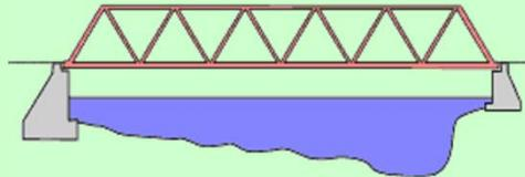
The **Warren** truss is perhaps the most common truss for both simple and continuous trusses. For smaller spans, no vertical members are used lending the structure a simple look. For longer spans vertical members are added providing extra strength.
