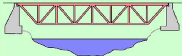
Warren trusses are typically used in spans of between 50-100m.
