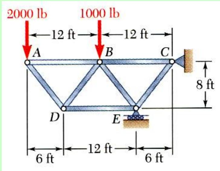
Using the method of joints, determine the force in each member of the truss.
