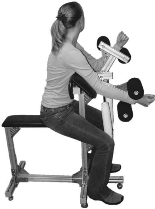
Fig. 1 Adjustable prototype configured like the original elbow flexion and extension exercise machine. The user sits with the upper arms resting against the elbow pads, and operates the machine arms in cyclic, reciprocal elbow flexion and extension motion as fast as possible against the hydraulic cylinder resistance.
