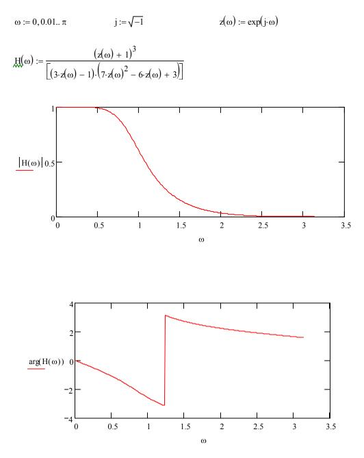
Example 3. In designing FIR filter one approach is to use truncation (windowing) and finite delay of the ideal (desired) impulse response function. For the ideal digital lowpass filter given as  $H_d(\omega) = 1$  for  $-\omega_c \le \omega \le \omega_c$  one gets the desired impulse response
