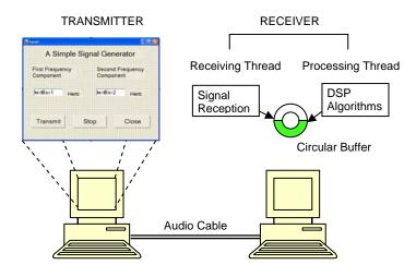
Figure 1. A platform that evaluates computational efficiency of DSP implementation.
