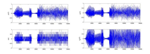
Figure 2. MATLAB example of quantization effect.
