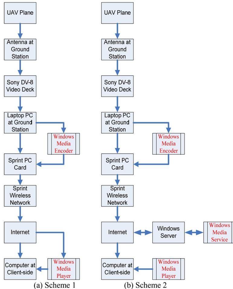
Figure 10 Block Diagrams of UAV Data Communication Links
