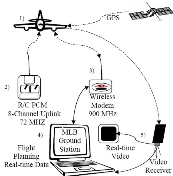
Figure 3 BAT III Communication System
