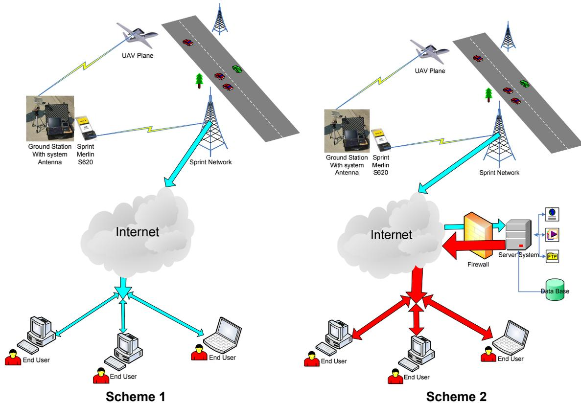
Figure 8 UAV Data Communication Link
