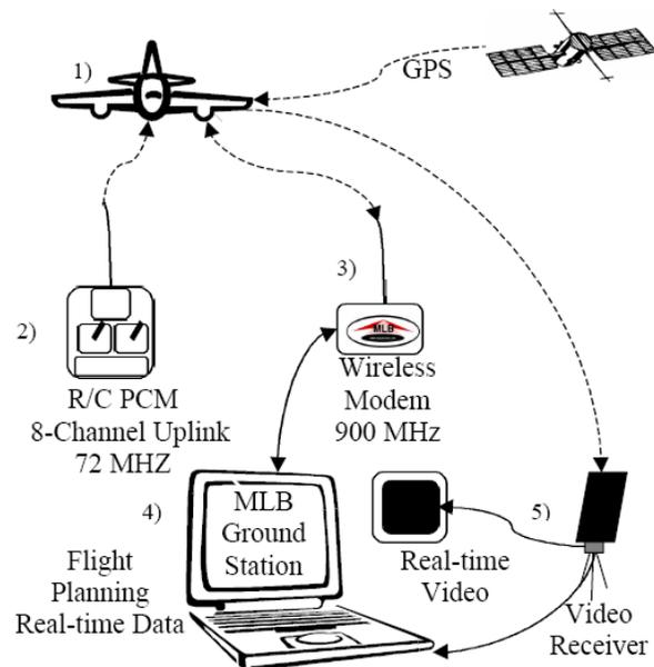
Figure 3 BAT III Communication System
