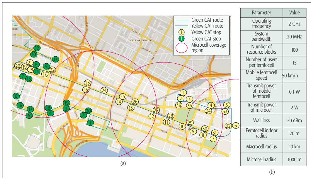
Figure 5. Simulation Scenario: a) Perth, Australia Central Area Transit (CAT) bus scenario; b) simulation parameters.
