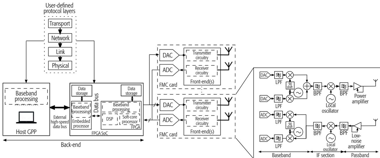
**Figure 1.** Generic software-defined radio architecture. Static analog transmit/receive circuitry (front-end) is interfaced with programmable hardware processing platforms (back-end) through ADCs/DACs. Analog-to-digital converters (ADCs)/digital-to-analog converters (DACs) and analog front-end radio circuitry may be featured under the same compact card, referred to as an FPGA mezzanine card (FMC).
