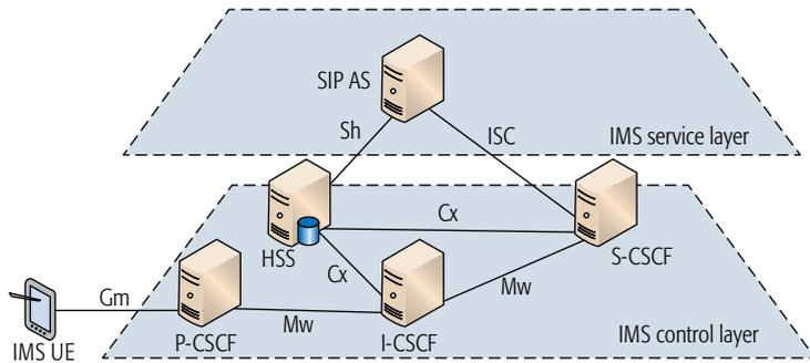
Figure 1. Simplified IMS architecture.
