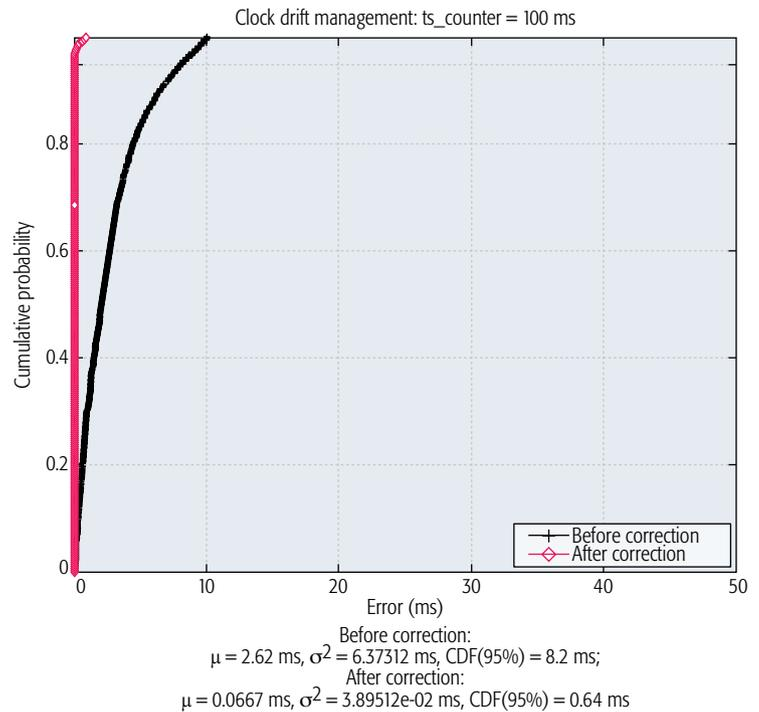
**Figure 3.** Clock drift management. There is one order of improvement in synchronization accuracy after compensating for clock drift, at both the average and 95 percent probability levels.
