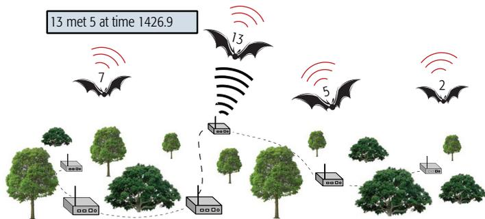
**Figure 1.** Conceptual scenario for bat tracking in the wild: stationary ground nodes are used to localize and track bats based on emitted beacon messages. The mobile nodes are also used to monitor encounters and download this data to the ground network to increase the observation range beyond the ground station area.
