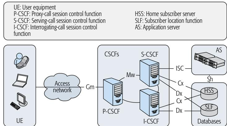
Figure 1. Simplified overview of the IMS architecture.
