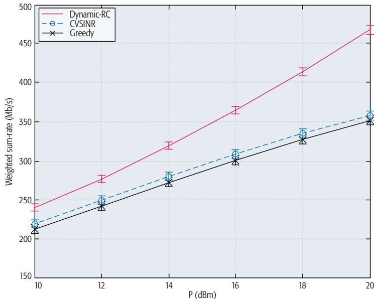
**Figure 6.** Improvement in downlink weighted sum rate (megabits per second) vs. RRH transmission power (dBm) of a C-RAN system employing dynamic clustering and cooperative beamforming. The competing strategies considered are dynamic-RC [15], a user-centric dynamic radio cooperation scheme; CVSINR, a user-centric heuristic clustering scheme with clustered virtual SINR beamforming; and greedy, a non-overlapping clustering scheme with zero-forcing beamforming.
