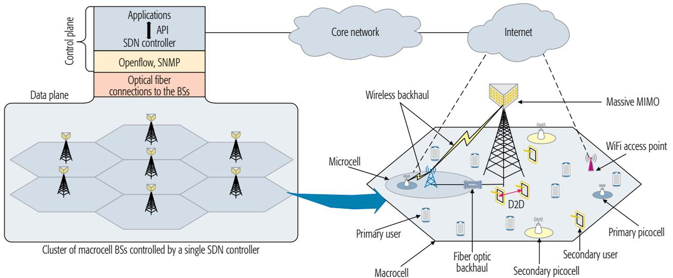
Figure 1. Software-defined 5G HetNet architecture that supports HSA. The macrocell BSs are directly connected to the controller, while the BSs of the smaller cells connect with the macrocells through a reliable backhaul link.
