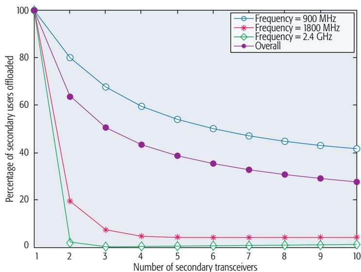
**Figure 7.** Percentage of secondary users offloaded from the primary network as a function of the number of secondary transceivers within the network.
