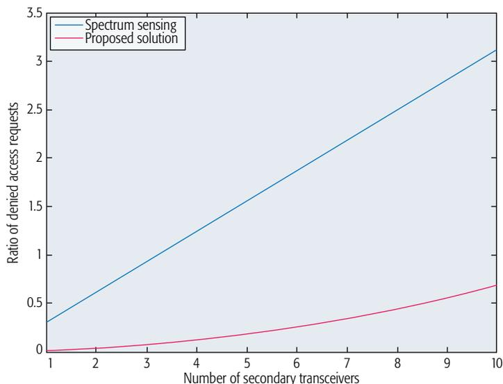
**Figure 6.** Average number of denied spectrum access requests as a function of the number of secondary transceivers within the network. The figure emphasizes the fact that the proposed resource management algorithm improves spectrum utilization by accommodating a larger number of secondary users.
