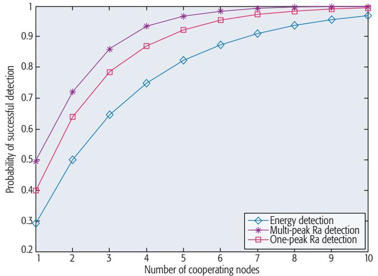
Figure 4. Probability of successful detection vs. the number of cooperating nodes. The figure highlights the fact that cooperative spectrum sensing requires a large number of cooperating nodes in order to achieve acceptable levels of performance.
