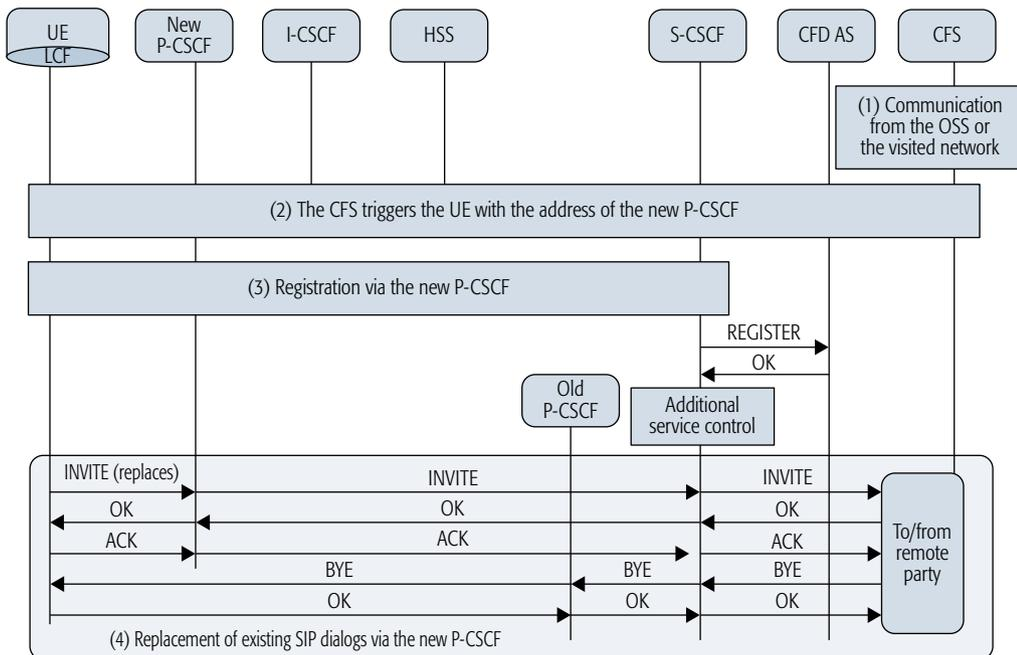
The operator may instruct the LCF to delay the replacement of each SIP dialog established by the terminal to a given deadline. This would allow distributing over time the signaling load corresponding to dialog replacement procedures, and even reducing this load by allowing the dialog to be terminated by the end user, via the old P-CSCF, before the deadline.
