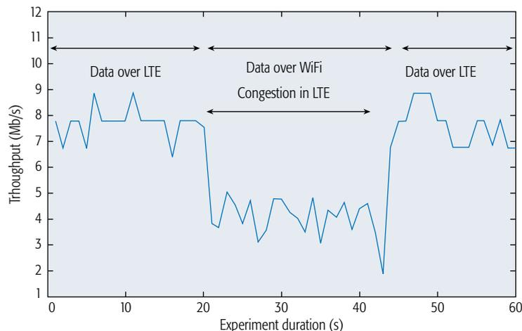
Figure 6. SDA data offloading performance.
