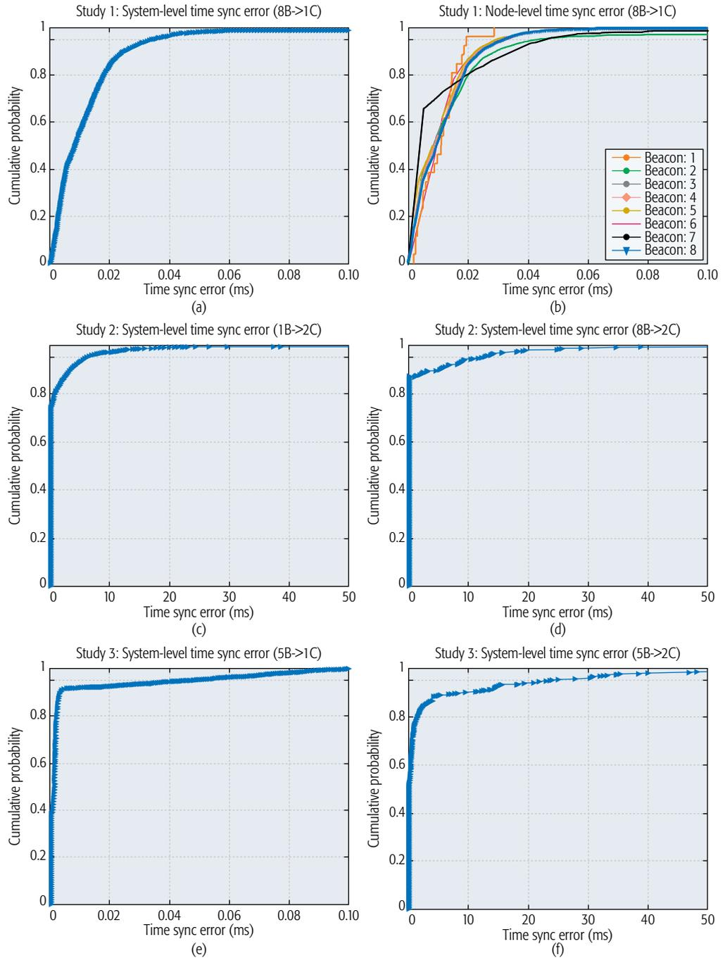
**Figure 4.** Performance of *CheepSync*. a) many-tx-to-one-rx:  $\mu = 8 \mu\text{s}$ , CDF(95 percent) = 0.04 ms; b) many-tx-to-one-rx; c) one-tx-to-many-rx scenario:  $\mu = 10 \mu\text{s}$ , CDF(95 percent) = 5 ms; d) many-tx-to-many-rx scenario:  $\mu = 10 \mu\text{s}$ , CDF(95 percent) = 10 ms; e) many-tx-to-one-rx scenario:  $\mu = 12 \mu\text{s}$ , CDF(95 percent) = 0.04 ms; f) many-tx-to-many-rx scenario:  $\mu = 10 \mu\text{s}$ , CDF(95 percent) = 22 ms.
