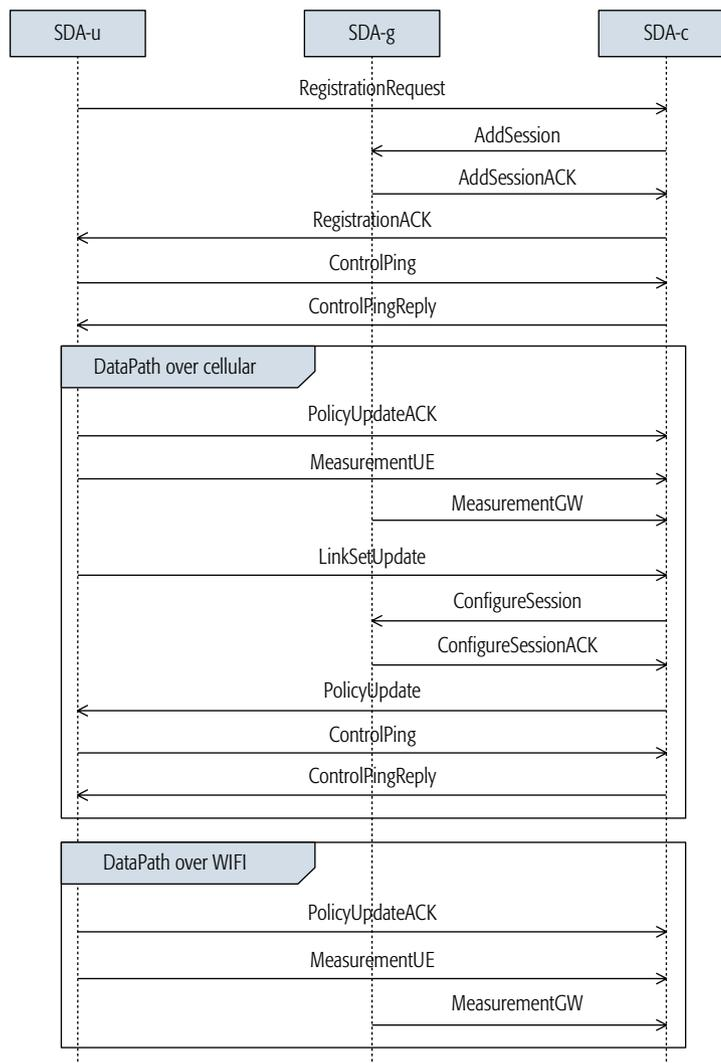
Figure 3. Sequence diagram for offloading.
