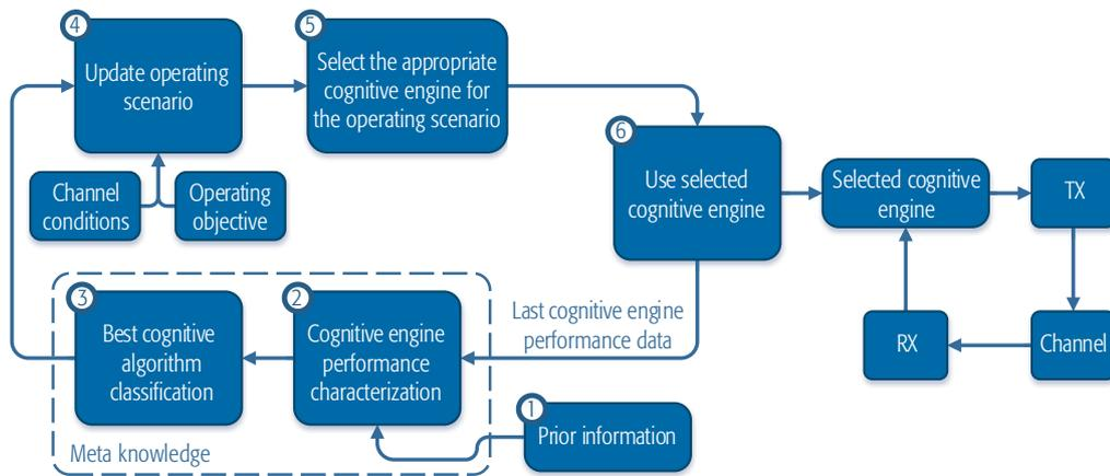
Figure 2. The metacognitive engine operation graph.
