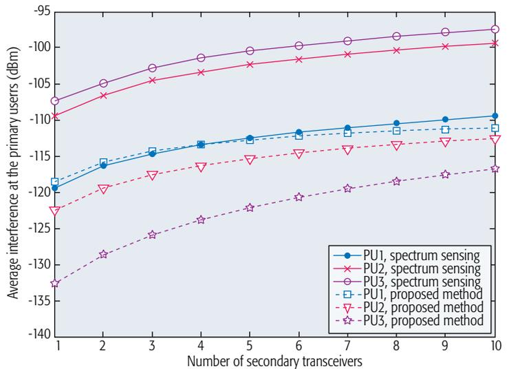
Figure 5. Average interference imposed on the PUs as a function of the number of secondary transceivers within the network. The figure shows that database-based spectrum management significantly outperforms spectrum-sensing-based resource management algorithms.
