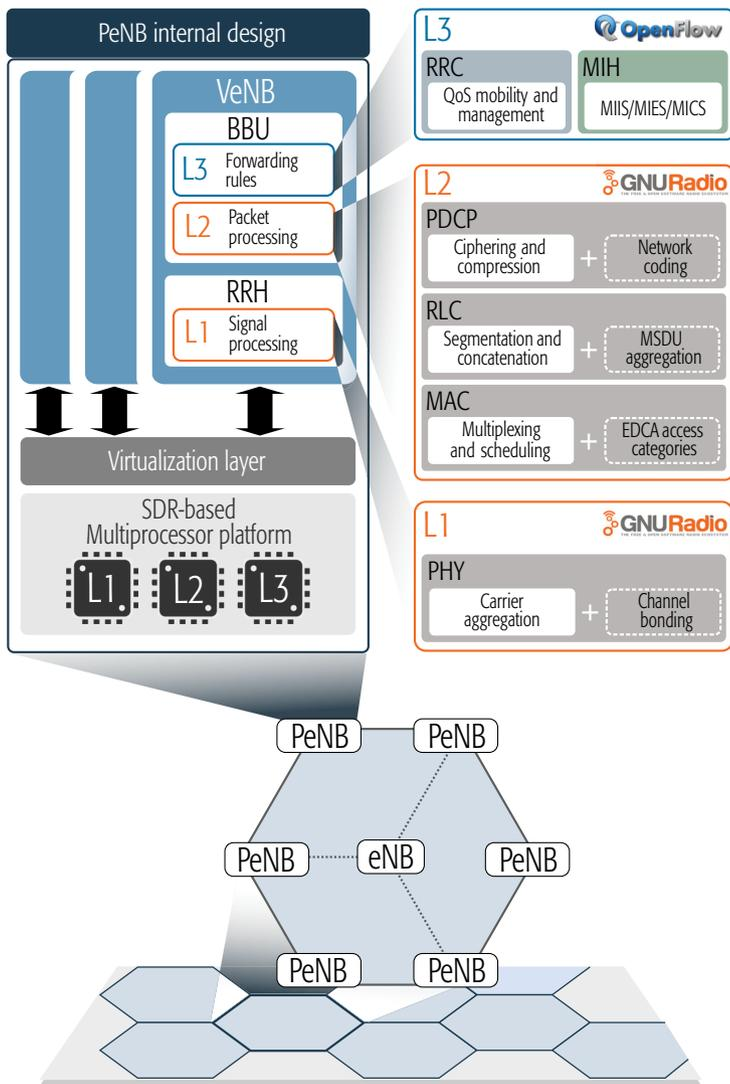
Figure 5. Internal design of PeNBs.
