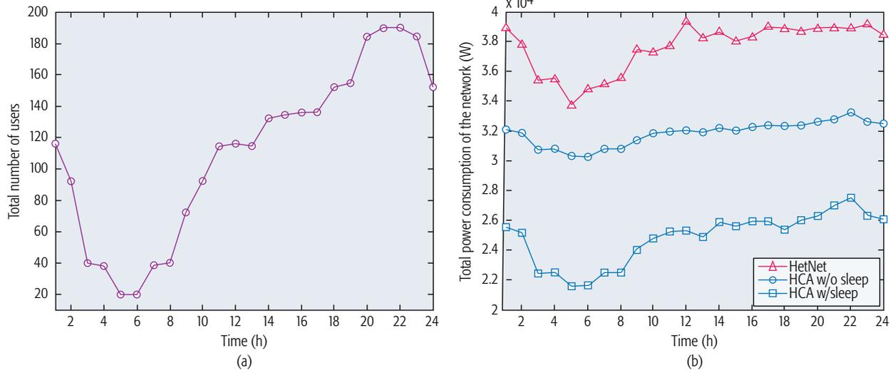
Figure 2. Simulation comparison of the network power consumption: a) average total number of users in the network for each hour; b) average total network power consumption for each hour.
