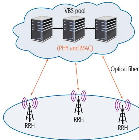
**Figure 1.** Cloud radio access network architecture, where the base stations are physically unbundled into virtual base stations and remote radio heads. Virtual base stations are housed in centralized processing pools and can communicate with each other at gigabit-per-second speeds.
