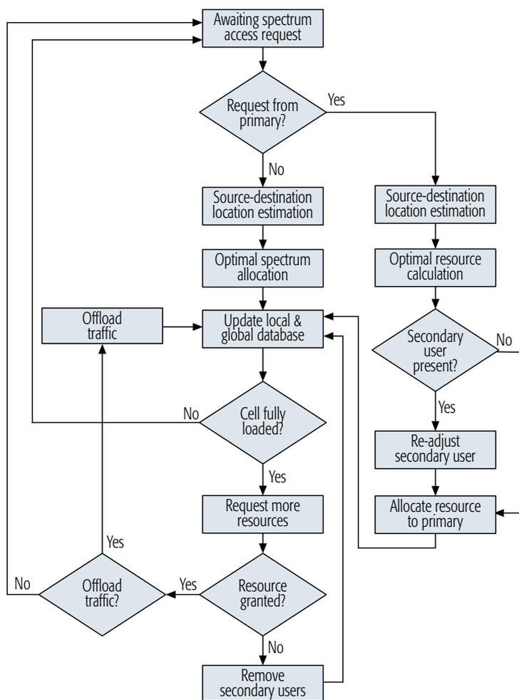
Figure 3. Resource management process at the BS. The proposed algorithm minimizes the dependence on spectrum sensing by relying on database assisted spectrum management.
