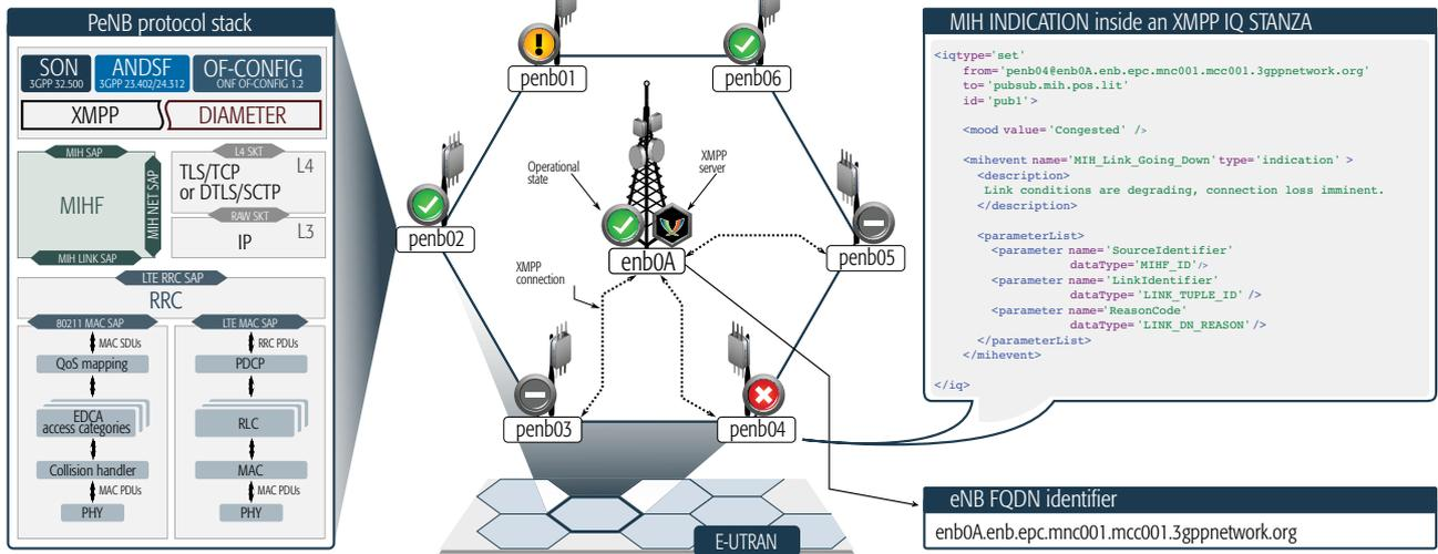
Figure 4. An instance of PeNBs deployed within the coverage area of an eNB.
