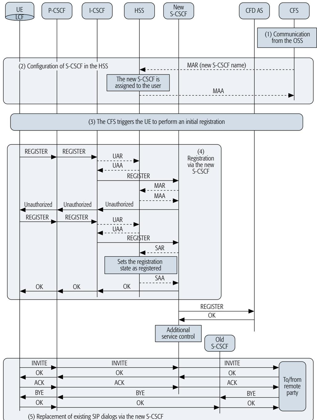
Figure 4. IMS procedures to change an S-CSCF allocation.
