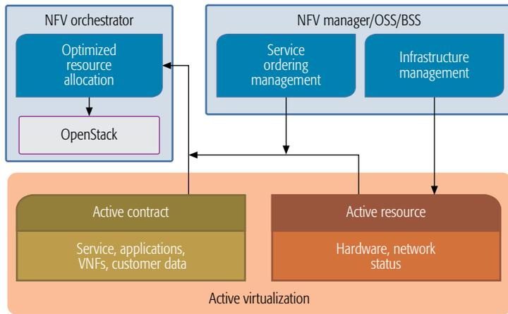
Figure 2. CloudNFV Architecture.
