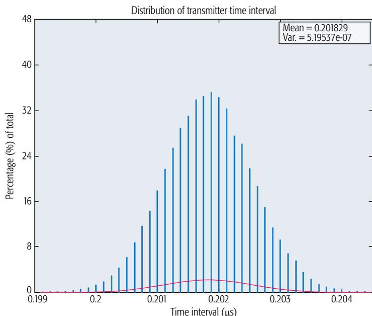
**Figure 2.** Transmitter side timestamping characteristics. Histogram showing the distribution of transmitter time interval recorded for 35,000 broadcast packets, grouped into 1  $\mu\text{s}$  buckets. The curve is a plot of the best fit Gaussian parameters with  $\mu = 0.201828 \mu\text{s}$  and  $\sigma^2 = 5.19537e-07 \mu\text{s}$ .
