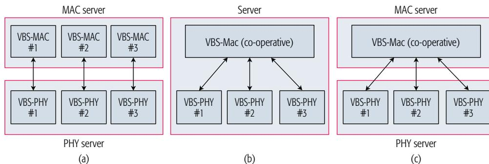
**Figure 4.** Split-VBS architectures: a) One-to-One mapping between PHY and MAC (different servers); b) Many-PHY-to-One-MAC (one server); c) Many-PHY-to-One-MAC (different servers). Note that the architectures in (a) and (c) (multi servers) can exploit the heterogeneity in datacenter server hardware.
