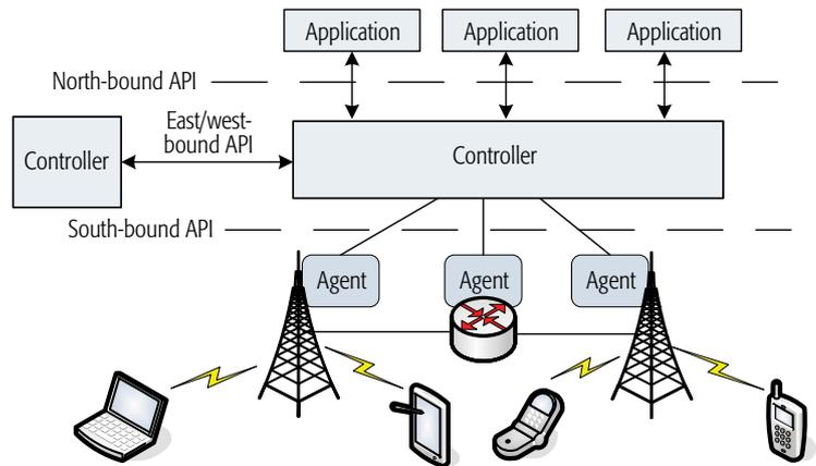
Figure 2. The conceptual architecture of SDWN.
