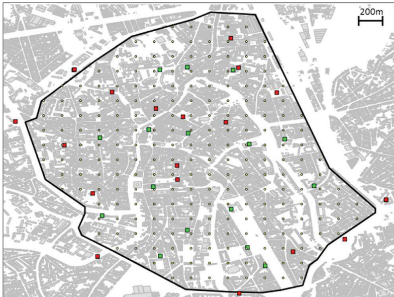
Figure 4. The selected suburban area of 6.85 km 2 in Ghent, Belgium. Users are located on the yellow dots; squares indicate base station (BS) sites. As an illustration of the sleep mode principle, the active and inactive BSs for a simulation with 70 percent available power and random user distribution are colored green and red, respectively.
