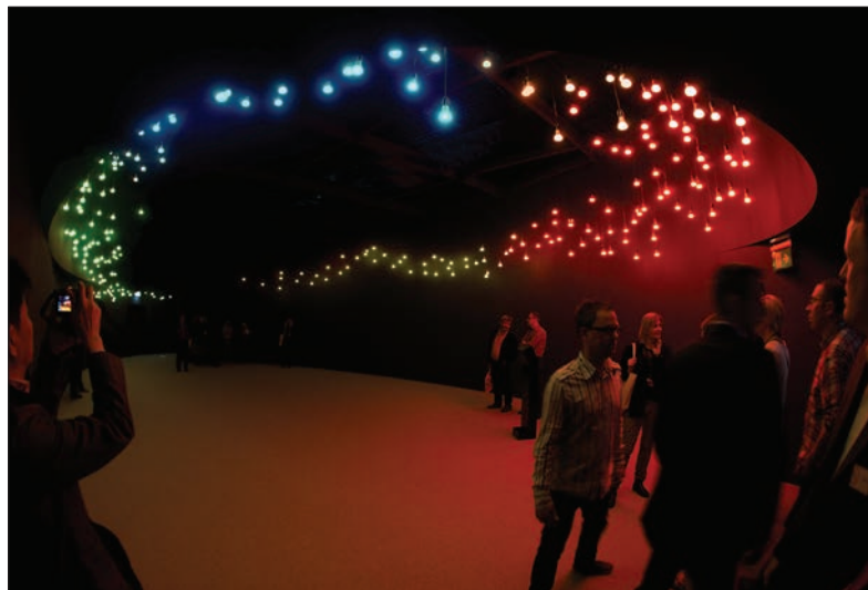
Figure 2. 300 Philips HUE lamps in a dense ZigBee network shown at the 2014 Light and Building Fair in Frankfurt.
