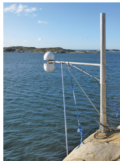
[FIG3] When a satellite passes overhead, the GNSS tide gauge uses signals from the satellite and signals reflected off the sea surface to measure the current sea level. (Photo courtesy of Onsala Space Observatory/J. Löfgren.)
