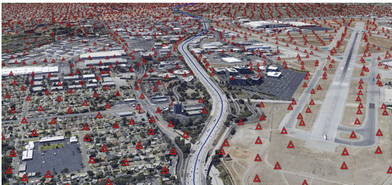
[FIG2] An aerial view of Long Beach, California, showing a portion of the 5,300-geophone network. Interstate 405 runs through the photo's center; a Long Beach Airport runway is on the right. (Photo courtesy of Scripps Institution of Oceanography at the University of California at San Diego.)
