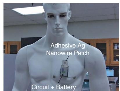
**FIGURE 2.** North Carolina State University researchers have developed a wearable, wireless sensor that can monitor a person's skin hydration to detect dehydration before it can begin posing health issues.
