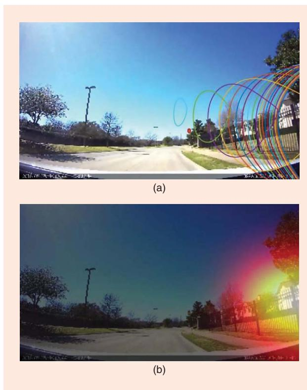
**FIGURE 7.** This visual saliency map was created with the probabilistic model and shows (a) the estimation of confidence regions for different distances from the car and (b) an aggregation of the results projected on the road camera. The saliency map characterizes driver visual attention.
