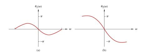
$\begin{array}{l} \text{Min-phase: } \angle H(\pi) - \angle H(0) = 0 \text{; Max-phase:} \\ \angle H(\pi) - \angle H(0) = \pi. \end{array} \\ \text{Note: For real-valued impulse responses, } \angle H(e^{j0}) = \angle H(0) = 0. \end{array}$
