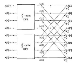
G(k) is an (N/2)-point DFT of even samples x(2r); H(k) is an (N/2)-point DFT of odd samples x(2r+1).
