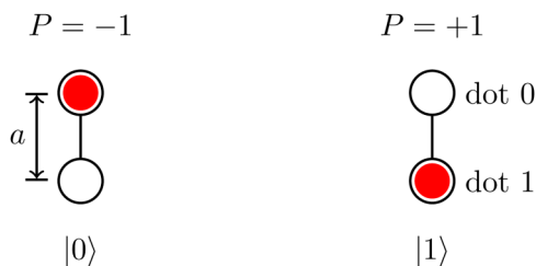
FIG. 1. Localized electronic states of a molecular double quantum dot (DQD) system provide the two classical states of a qubit. Black circles represent the two quantum dots, and a connecting bar indicates a tunneling path. A red disk represents the mobile electron.
