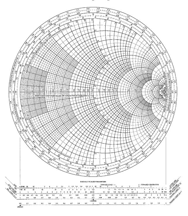
**PROBLEM 4 (20 points):** Use single-stub impedance matching techniques with the Smith Chart on the following page to provide  $Z_{in} = 50 \Omega$ . Use an open-circuit stub and find d and l in terms of  $\lambda$ . Use  $Z_0 = 50 \Omega$  for all transmission lines.
