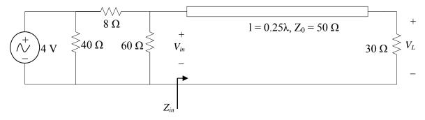
(a) Find  $Z_{in}$ , the input impedance to the transmission line (5 points).
