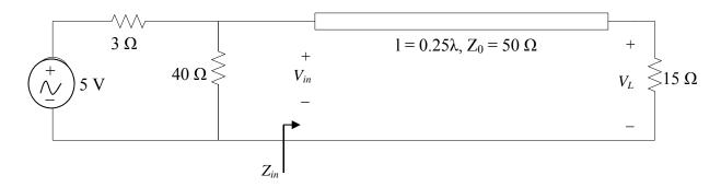
(a) Find  $Z_{in}$ , the input impedance to the transmission line (5 points).
