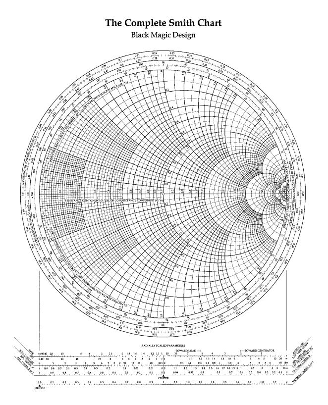
**PROBLEM 4 (20 points):** Use single-stub impedance matching techniques with the Smith Chart on the following page to provide  $Z_{in} = 50 \Omega$ . Use an open-circuit stub and find d and l in terms of  $\lambda$ . Use  $Z_0 = 50 \Omega$  for all transmission lines.
