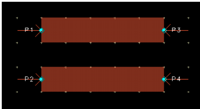
Figure 7. Coplanar waveguide line after placing ports at four positions.
