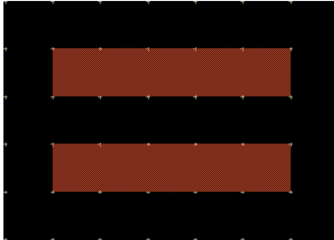
Figure 4. Slot version of a simple coplanar waveguide line.
