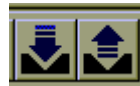
Figure 6. Buttons used to automatically “push into” a lower level schematic (right) or “pop out of” a lower level schematic (left).
