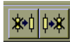
Figure 5. Buttons used to activate (left) and deactivate (right) elements in a schematic.
